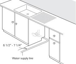
Use new hoses when connecting to the water supply. Do not reuse old hoses.
