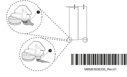
**4.** Remove the No. (4) screw from the radiation grill in the back of the product. Align the No. (1) bracket frame in the hole in the product and reassemble it using the No. (4) screw.
